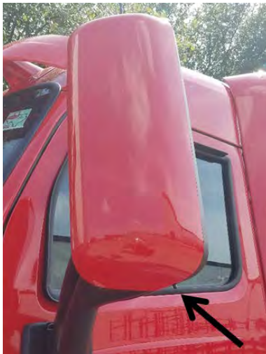
FIGURE 2-3: Aerodynamic Mirror OAT Sensor Location
