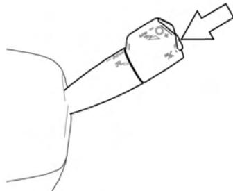
Pressing this button places the transmission in Manual mode. Manual mode allows the operator to select the gear (See [Upshifting and Downshifting](#) on page 29).
