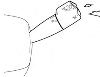
The transmission gear can be selected manually to accommodate the driving needs of the operator. The transmission mode must be in either Drive or Reverse to manually select the gear.
