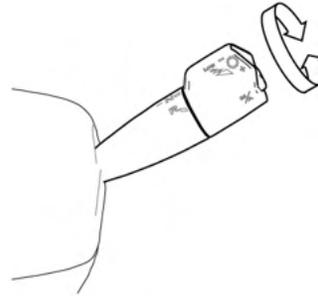
Select the transmission mode by rotating the shifter outer knob. There is a position for Drive (**D**), Neutral (**N**), Reverse (**R**). Rotating the knob to the Reverse (**R**) position while moving forward, or to the Drive (**D**) position while moving backward, will not change the transmission mode to those selections.
