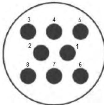
**Figure 6-7.** Cab Body Builder Connection 1 Pin Assignment
