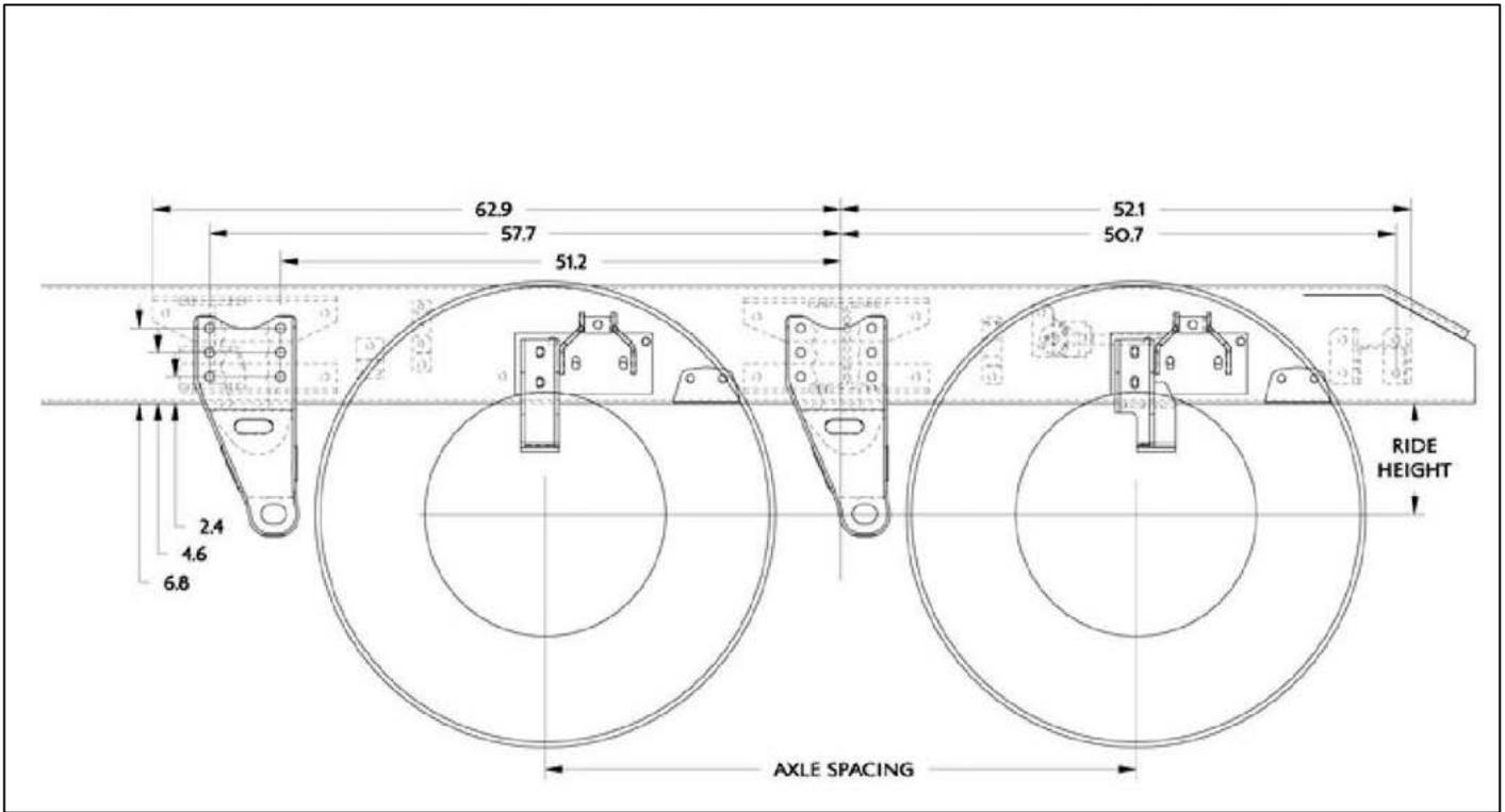
FIGURE 3-7. Neway ADZ 252 Frame Drilling (Dimensions In Millimeters)
