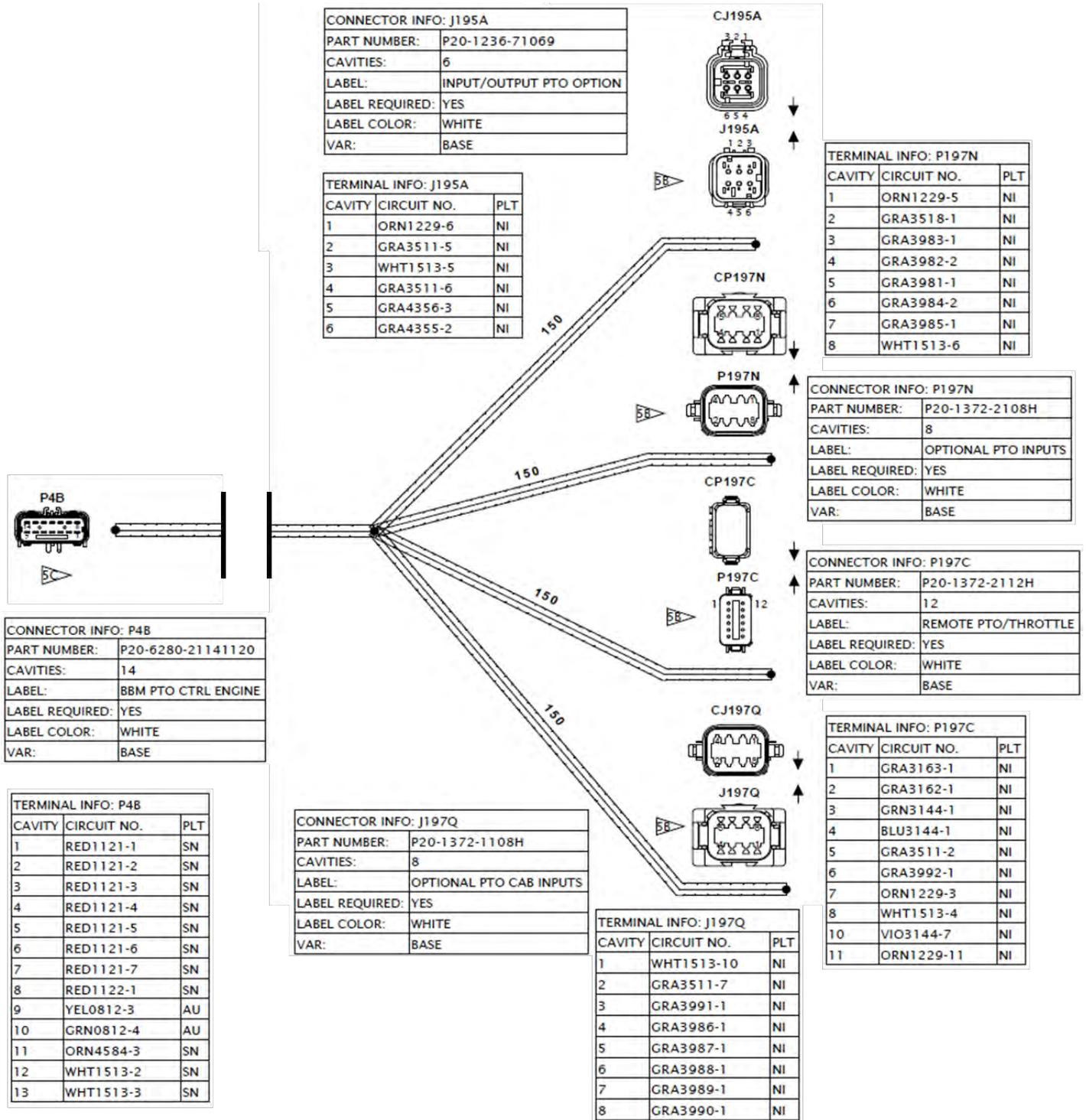
FIGURE 6-16. Body Builder Module Control Harness A92-6061
