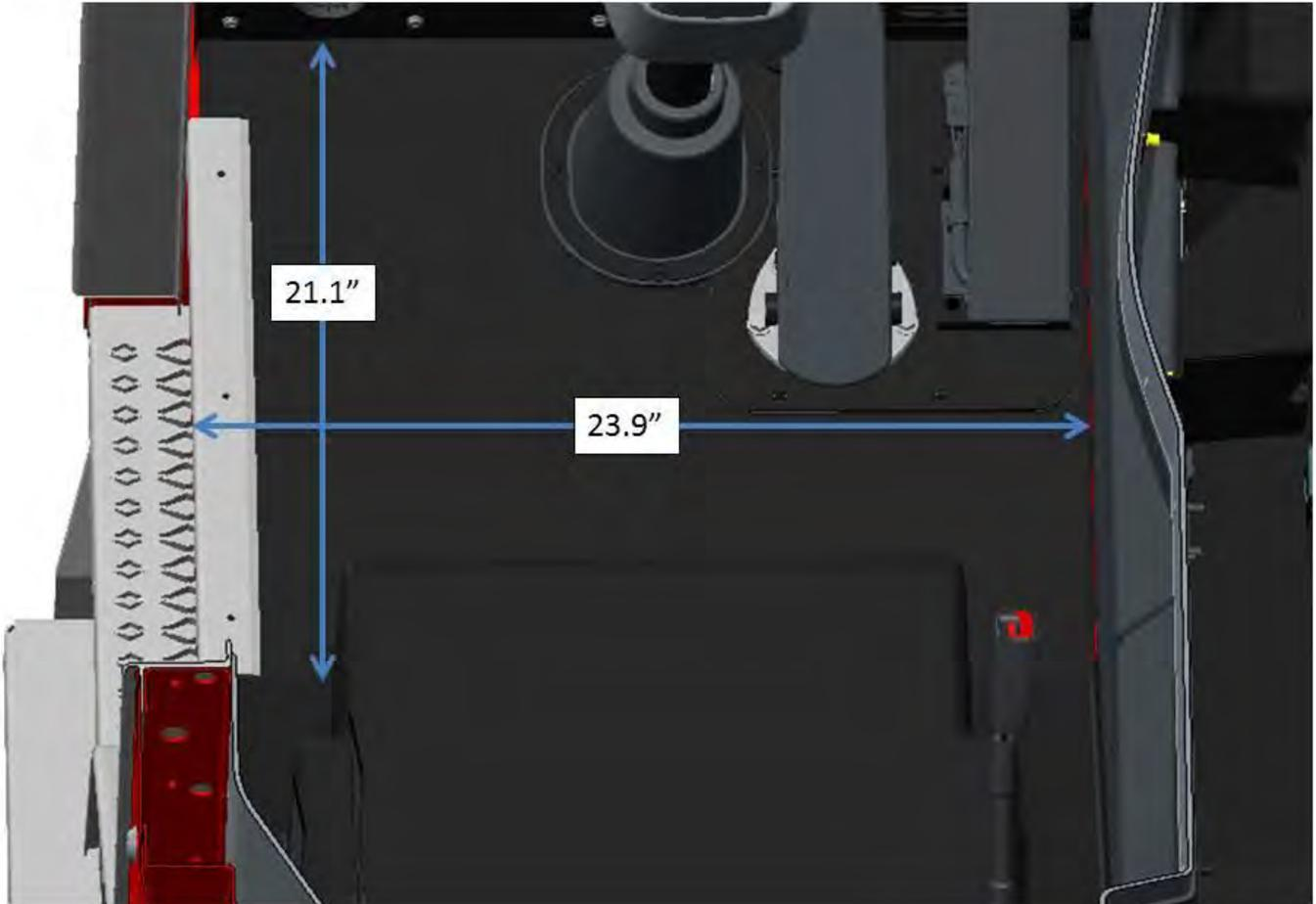
**FIGURE 3-6.** Floor Dimensions for LH Floor
