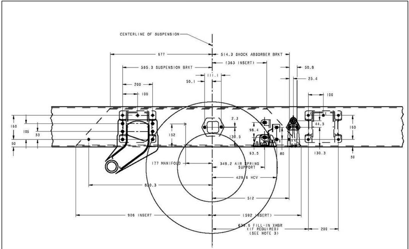
FIGURE 3-6. Reycos 102AR Frame Drilling (Dimensions In Millimeters)
