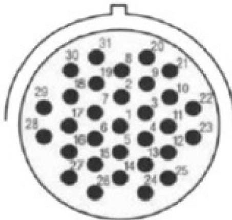
Figure 6-9. Cab Body Builder Connection 1 Pin Assignment
