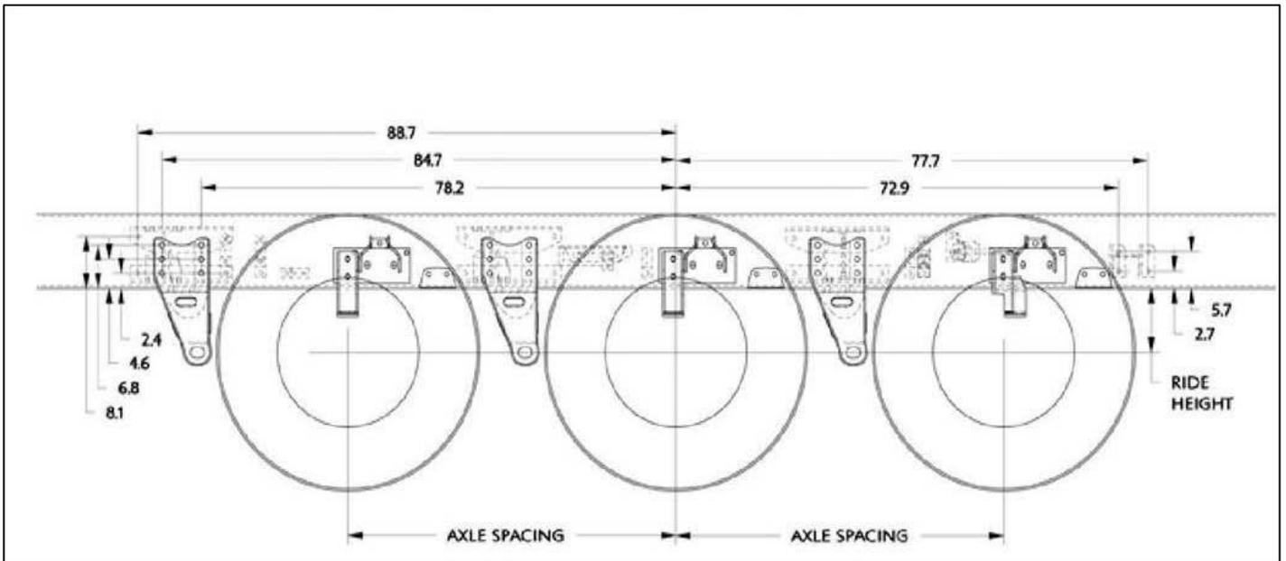
FIGURE 3-8. Neway ADZ 369/378 Frame Drilling (Dimensions In Millimeters)
