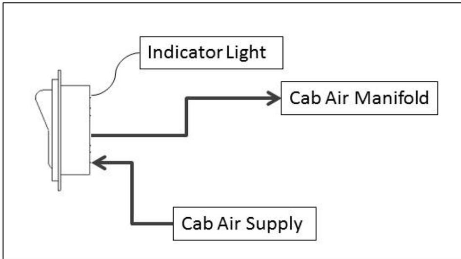
**FIGURE 7-8.** (1) Single acting PTO Controls Diagram
