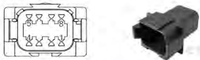
**FIGURE 6-19.** Customer Interface P197Q Connector – Pinouts
