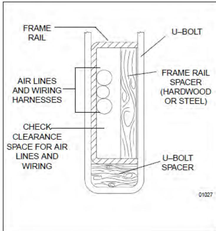
**FIGURE 4-10.** Clearance Space for Air Lines and Cables
