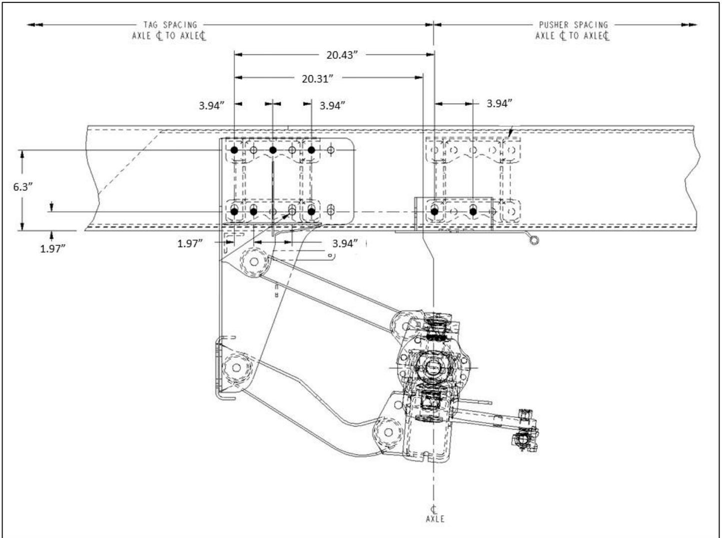
FIGURE 3-26. Watson-Chalin SL0893SSR or SL1093SSR Pusher or Tag
