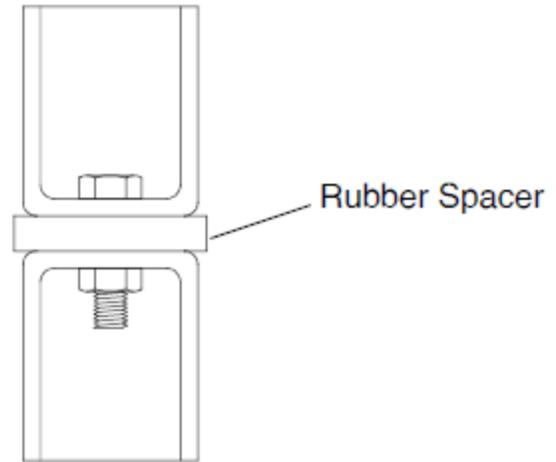
**FIGURE 4-5.** Mounting Brackets
