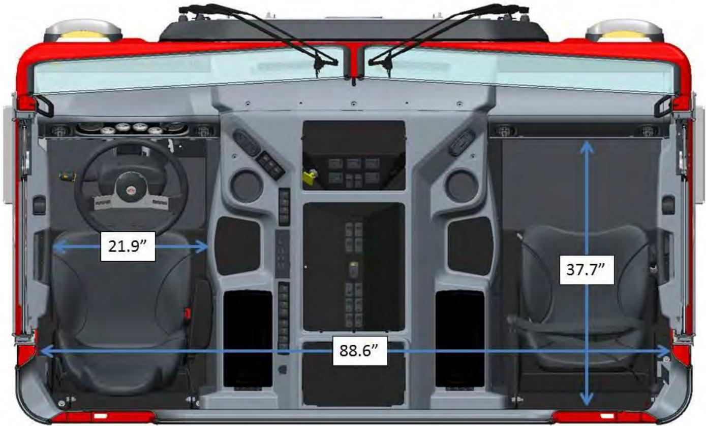
FIGURE 3-5. Top View of LH Steer Model
