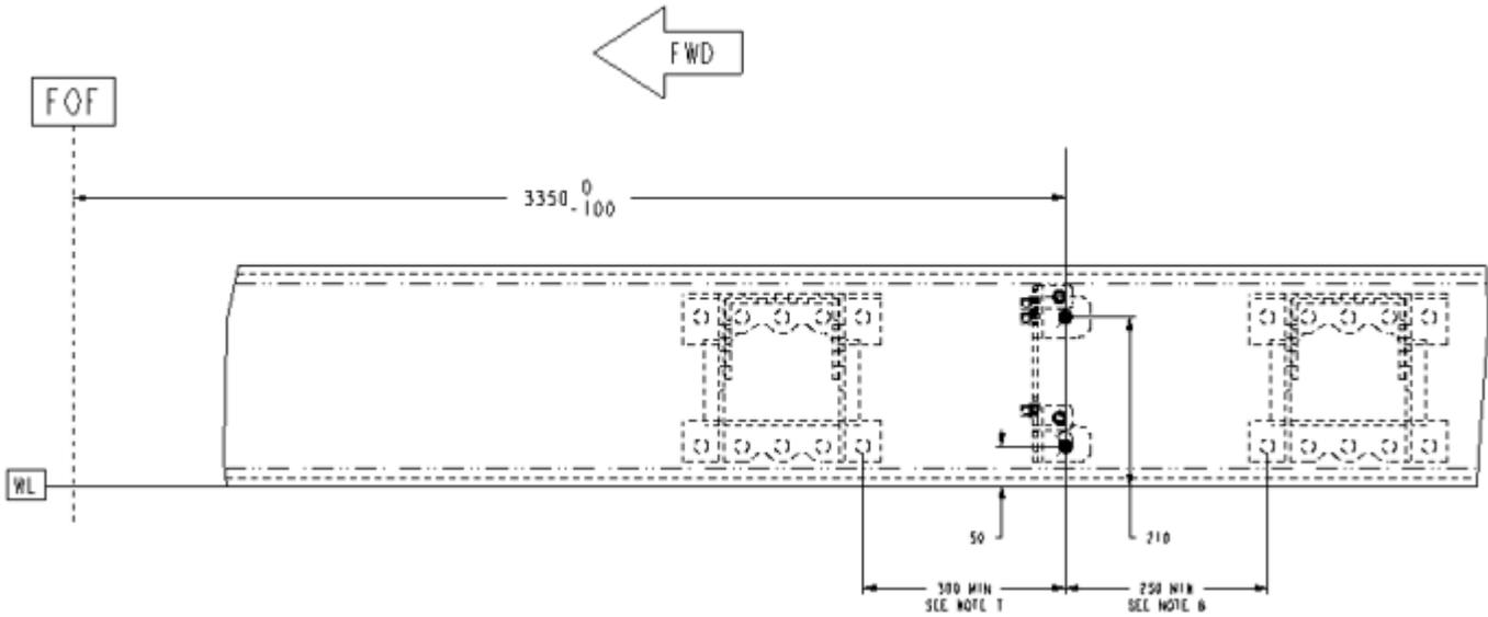
**FIGURE 7-13.** Optional Module Drilling Location for Bracket Installation
