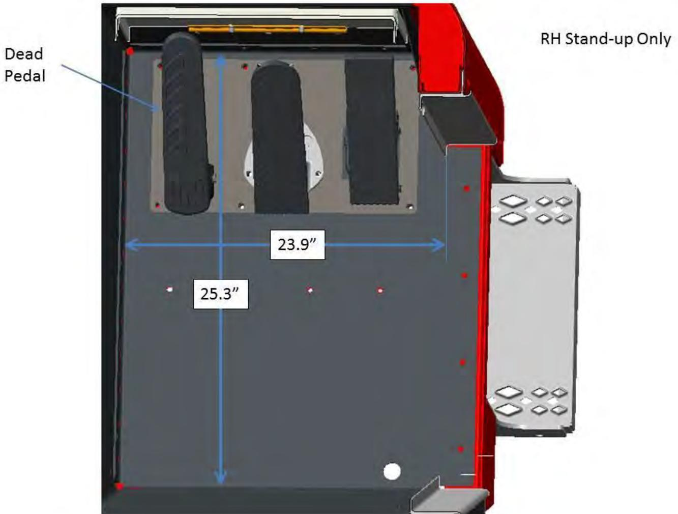
FIGURE 3-7. Passenger Floor RH Stand Up
