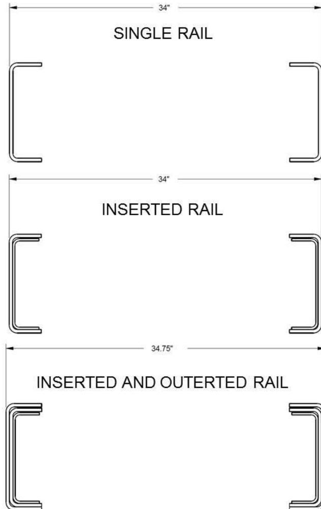
**FIGURE 3-8.** Frame Rail Configurations
