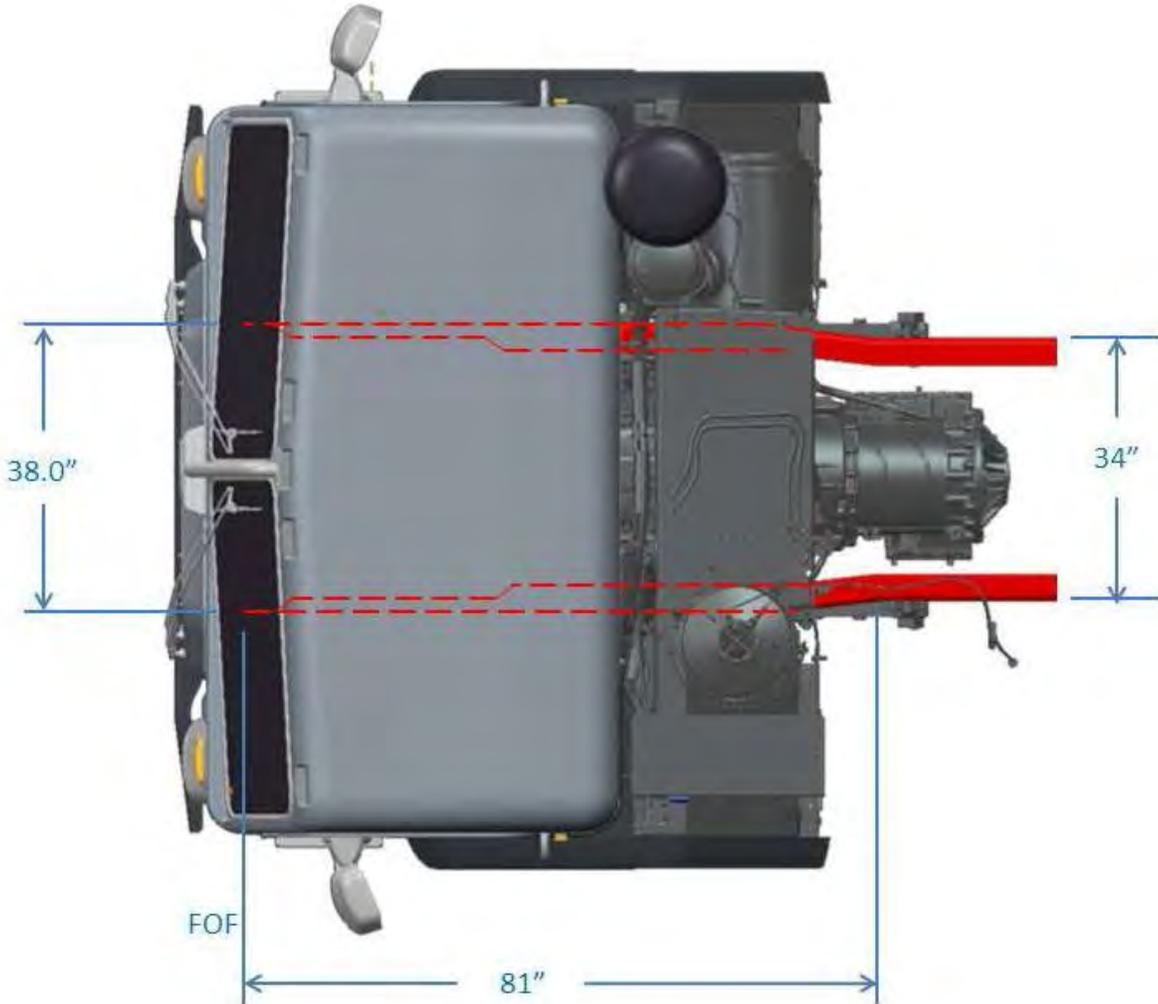
FIGURE 3-9. Model 520 Frame Rail
