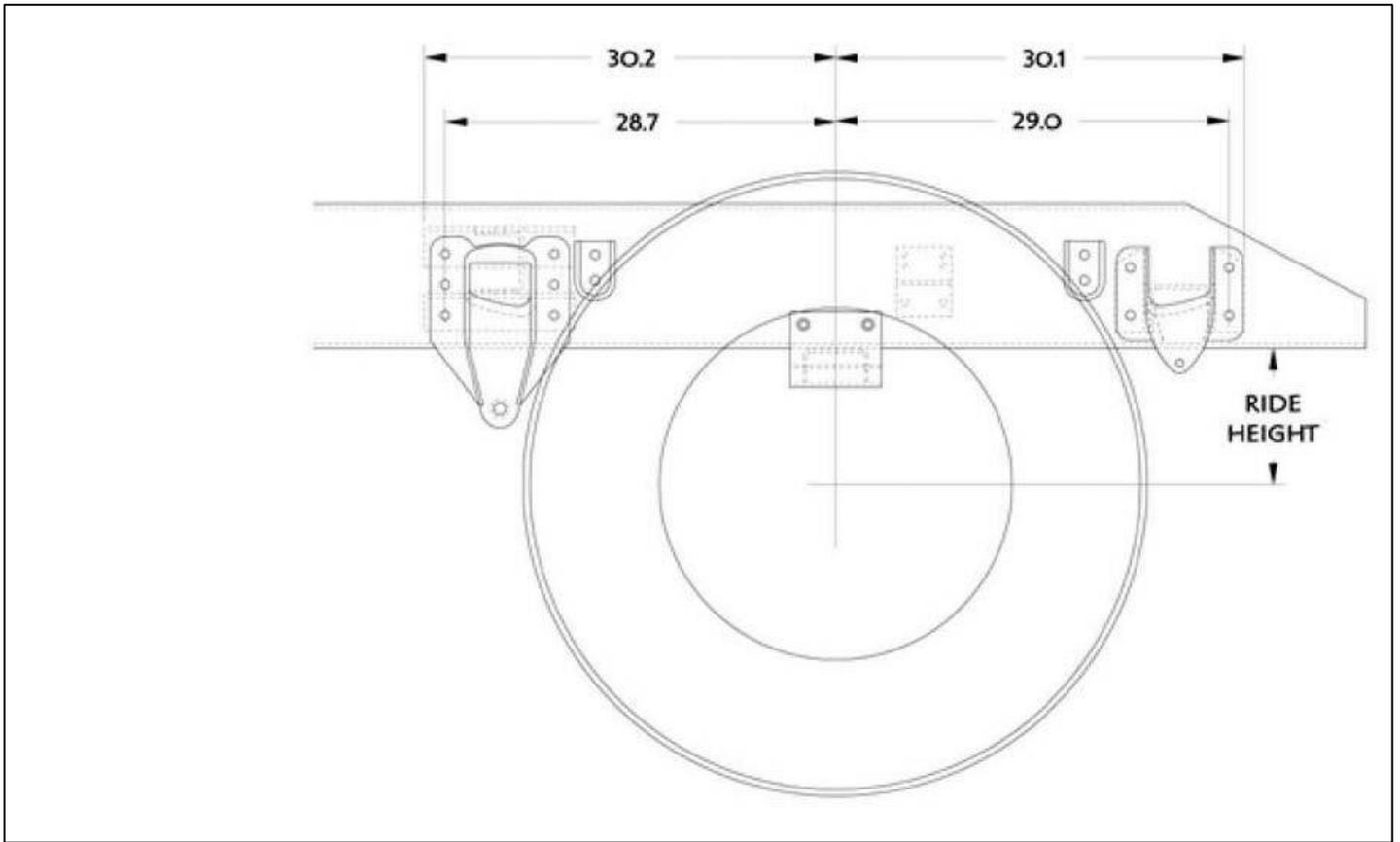
FIGURE 3-5. Reycor 79KB Frame Drilling (Dimensions In Millimeters)
