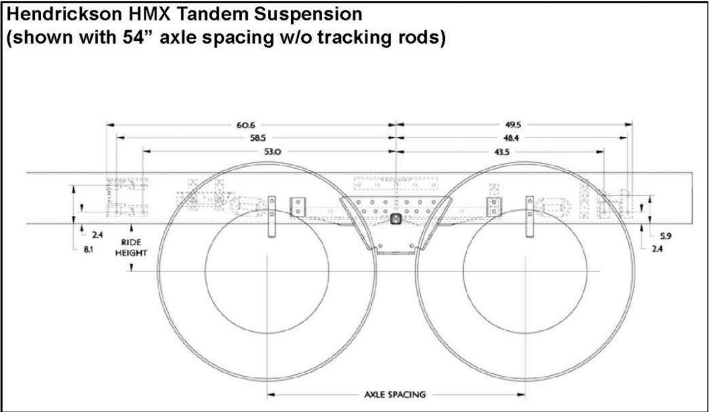
**FIGURE 3-15.** Hendrickson HMX Tandem Frame Drilling
