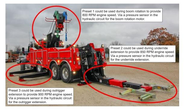
Figure 33: Custom Presets wiring at the P197n PTO optional connector
