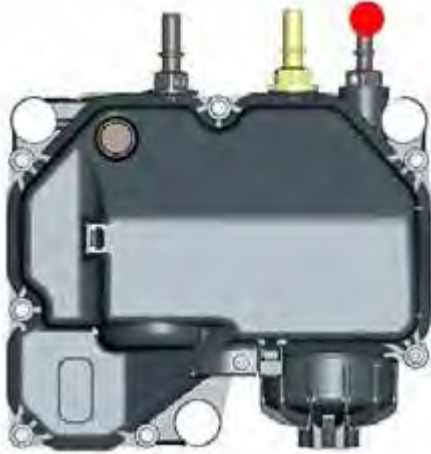
Figure 4-2 Measurement Location of DEF Supply Module (Pump)
