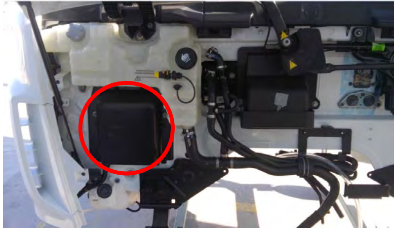
Figure 7-3.1 Electrical Junction Box Location
