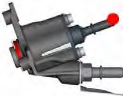
Figure 4-3 Measurement Location of DEF Dosing Module (Injector)
