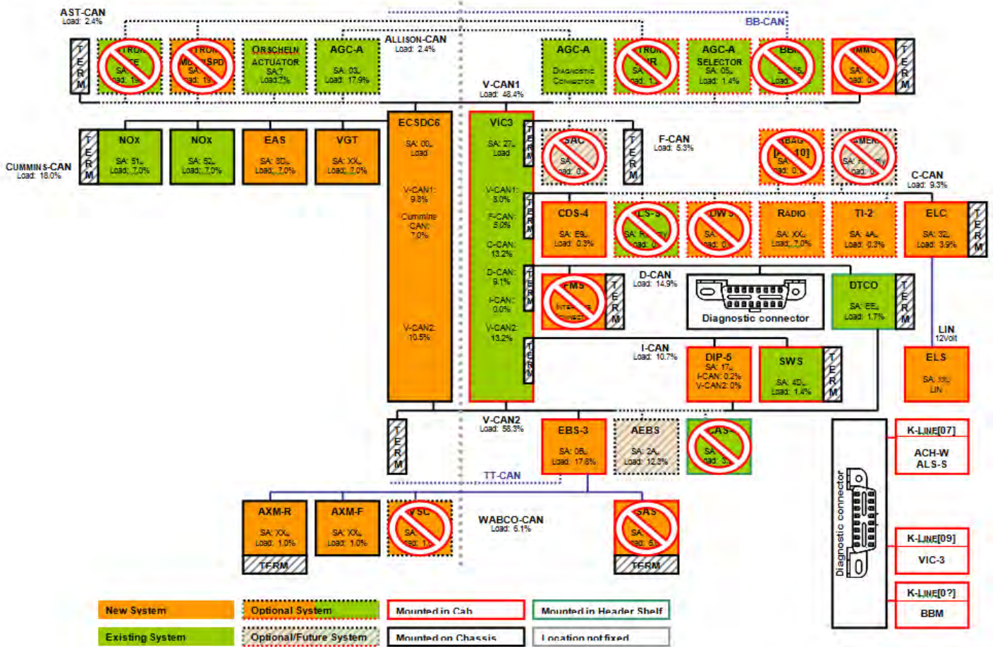
Figure 7-2 Data Bus Communication Architecture
