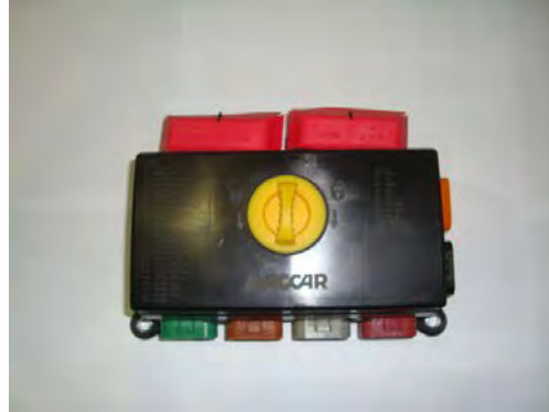
Figure 7.6.1 Pwer Distribution Center
