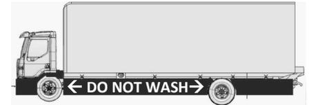
Avoid getting any part of the undercarriage wet, especially the areas where the battery systems and cables are housed.
