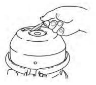
2. Remove the release stud assembly from the side pocket. Then remove the release nut and washer from the release stud.
