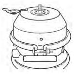
With a wrench, turn the release stud assembly nut until the compression spring is 90-95 percent caged. While turning, make sure that the pushrod (adapter pushrod, or service pushrod) retracts. DO NOT over-torque the release stud assembly. (S-camtype maximum: 50 lb-ft (68 N·m), Wedge-type maximum: 30 lb-ft (41 N·m)). The spring brake is now mechanically released.
