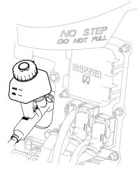
Visually inspect the clutch fluid from the reservoir. There are molded lines with the letters MIN to indicate minimum fluid level and MAX to indicate the maximum fluid level recommended for proper operation. Be sure to maintain the fluid between the MIN and MAX levels indicated on the plastic reservoir. If the fluid level repeatedly goes below the MIN line, then it is time to have your clutch adjusted or the hydraulic system inspected for service. To replace
