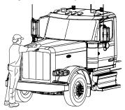
Tilt hood forward until it stops. When fully opened, the hood lock engages automatically.
